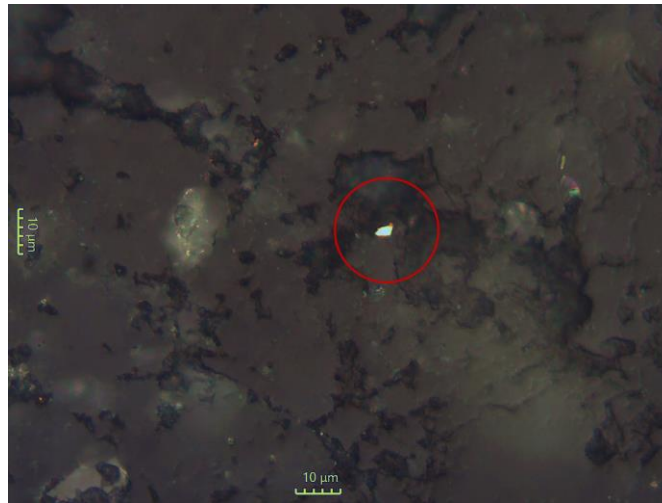
Photo 13-22: Sill Drum 13 - Liberated Grain of Yellow Sphalerite with Exsolution Bodies of Yellow Chalcopyrite – 500X RL
