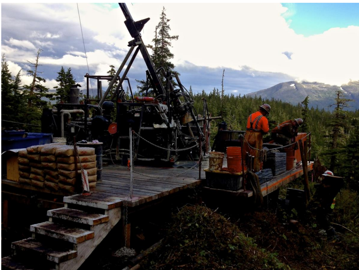
Photo 10-1: Typical Timberline Core Drilling Set Up
